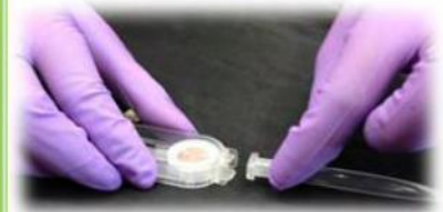
Step 4: Separate Reaction Tube from LYNX Plasma Separator
